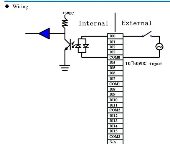
External Wiring (external connect with 0 ~ 50VDC, both positive and negative direction is OK)
